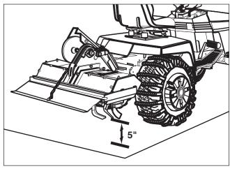
Figure 22. Lift Height Adjustment
